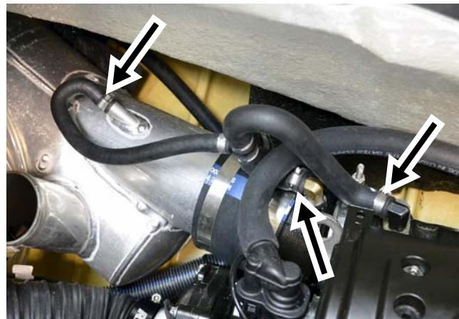
Loosen clamp securing water box exhaust pipe to exhaust manifold.
