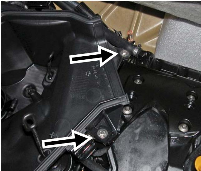
Squeeze outlet hose inside air intake silencer.
