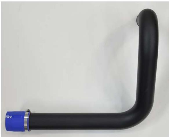
Install Aluminum Exhaust Tube at Rear Exhaust Outlet first and then Water Box.
